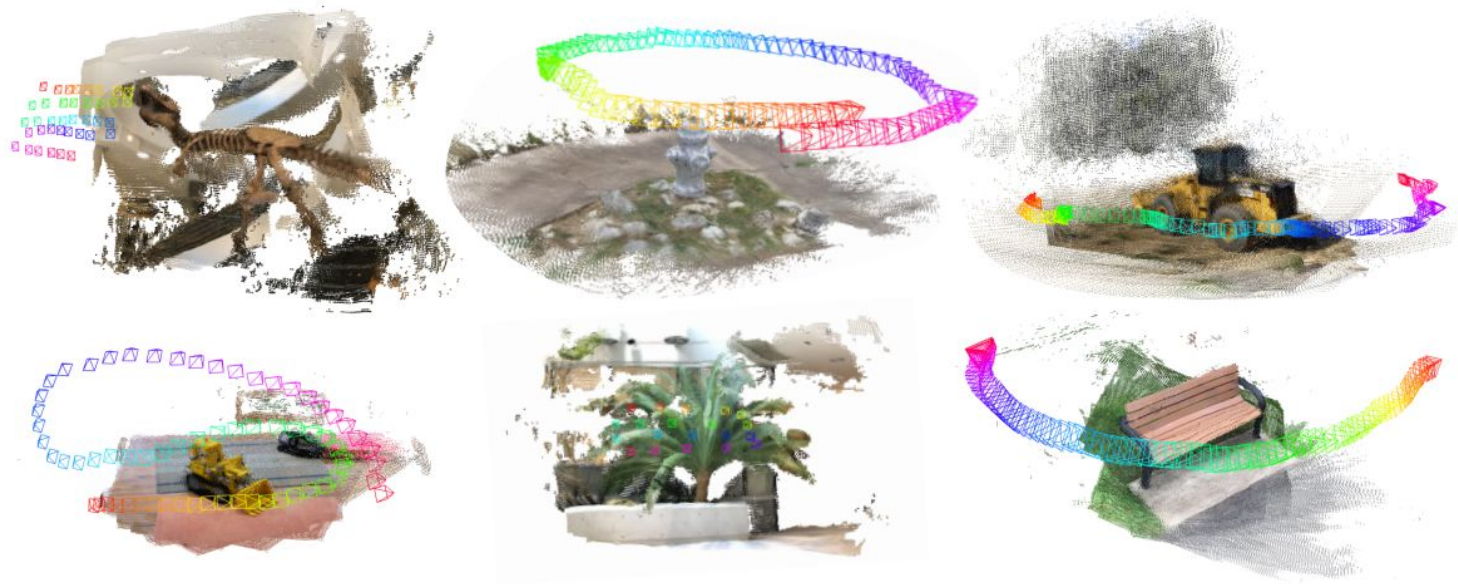
Fig. 7: Point Clouds Reconstructed by FlowMap. Unprojecting FlowMap depths using FlowMap's intrinsics and poses yields dense and consistent point clouds.
